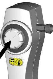
The High Flow system has a automatic push feature to continually dispense diluted chemical. There is a small plug with a lock symbol, when removed it allows the feature to operate. Push and twist the grey operating button clockwise to activate the feature. When the container is full push the operating button again to deactivate.
