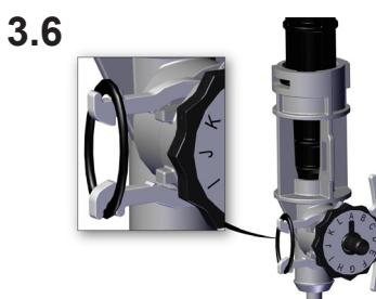
Rotate venturi body 2 anti-clockwise to release venturi body 1. Remove the 'O' ring and dilution clip. Replace the dilution clip and 'O' ring on the opposite side.
