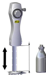
Screws are provided in the box, if using a bottle bracket set the height correctly.
