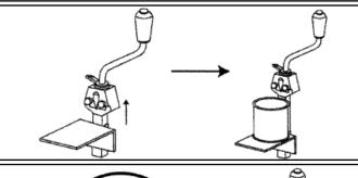
Back the rilsan lever (in an anti-clockwise direction) and lift.
