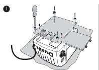
Unplug and place toaster on a soft cloth. Remove crumb tray and unscrew feet to remove the base plate
