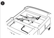
Loosen locking nuts on retaining plate using a 6.5mm spanner and slide back
