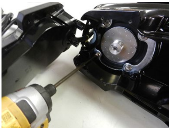
Fig. 28: Remove the 4 motor mount screws.
