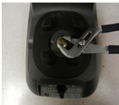
Fig.5: With Pliers, grasp the drive coupling.
