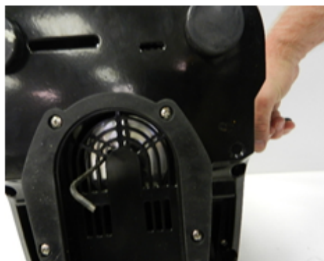
Fig.6: As shown, now turn the coupling with the pliers to spin the coupling off of the shaft while the output pulley is being held.
