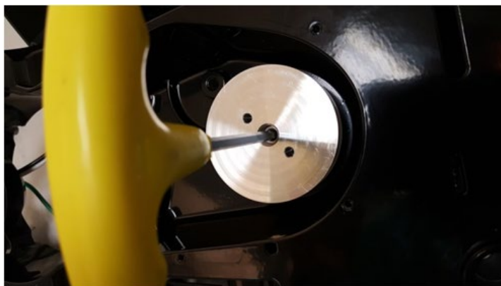
Fig.24: Insert a 5 mm hex key wrench and turn the screw clockwise to thread the output pulley off of the spindle.
