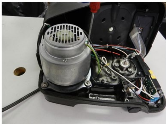
Fig. 27: Use a T20 Torx driver to remove the motor ground screw.
