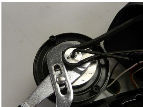
Fig. 29: Temporarily put the belt back on the motor pulley and hold with pliers while also using a 4mm allen wrench to turn the motor shaft counter-clockwise to remove the pulley.
