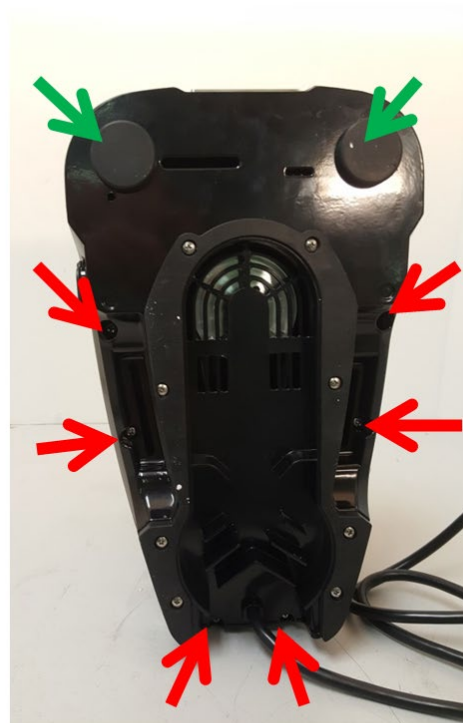
Figure 2: Remove 6 base screws (red arrows). At the green arrows, remove the rubber feet by simply pulling and twisting them out of the base.
