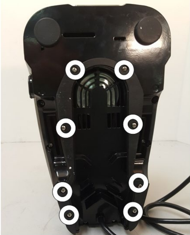
Fig. 21: Remove these screws in the base to get to the belt pulley area.
