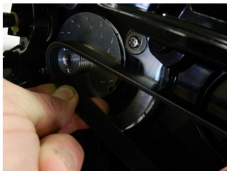
Fig.23: Carefully roll the drive belt off of the smaller pulley at the motor.
