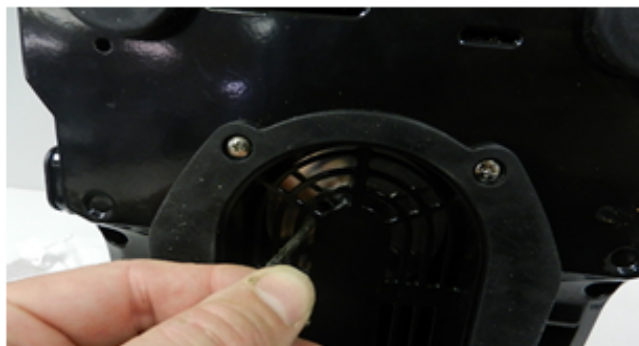
Fig. 4: Put a suitable tool, ( in this case, an 1/8 allen wrench is used), into the ribs of the base at the drive pulley. Align one of the holes in the pulley with the tool and insert it into the pulley.
