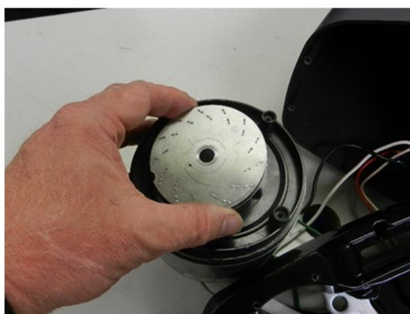
Fig.30: Once the belt pulley is removed, then remove fan off of the shaft.
