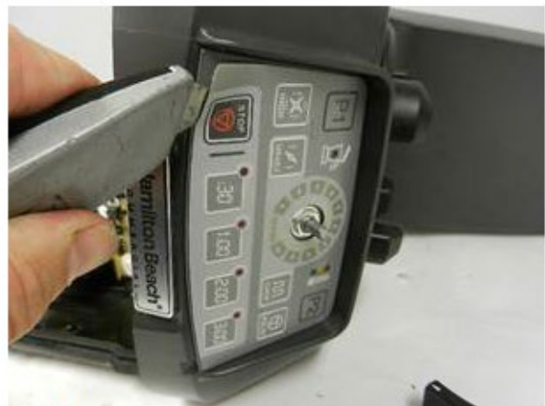
Fig. 34: With an utility knife, separate the adhesive backed Touchpad from the backing plate of the touchpad Assembly. Pull the old touchpad off. Replacement Is the reverse of these steps.
