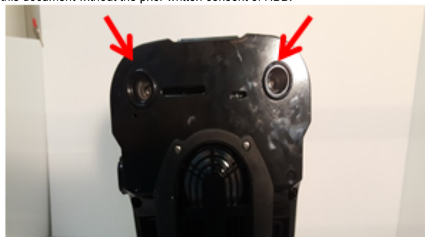
Figure 3: Once the 2 front rubber feet are removed from the base, 2 screws will be visible, remove these screws.
