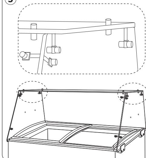
Step 5: Mount the top glass panel and fix it with the side panels with the joint assembly.
