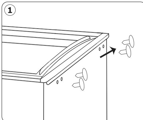
Step 1: Remove the protective caps from the sides of GM489/GM489.
