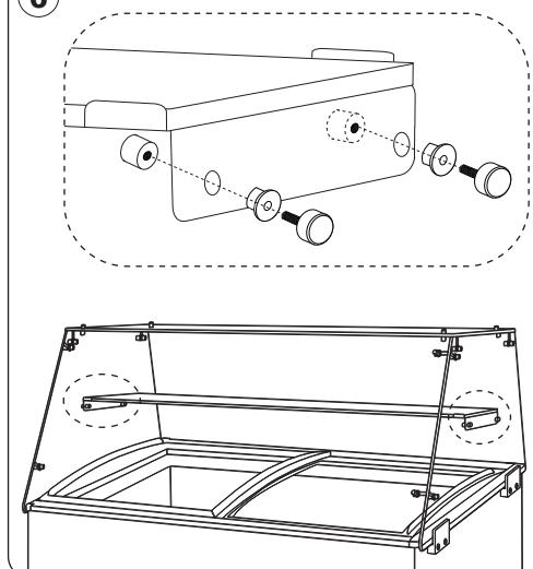
Step 6: Mount the glass shelf support with bolt assembly. Then put the glass shelf in place. Now the glass surround is mounted.
