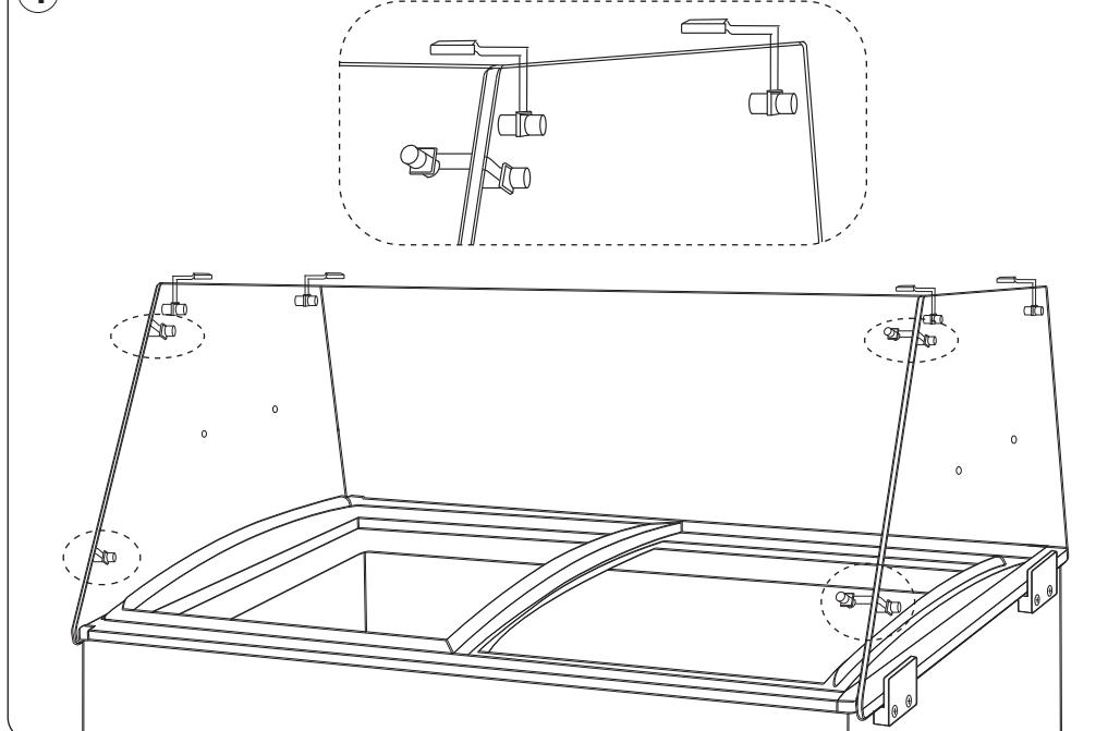
Step 4: Mount the front glass panel and fix it with side panels with the joint assembly.
