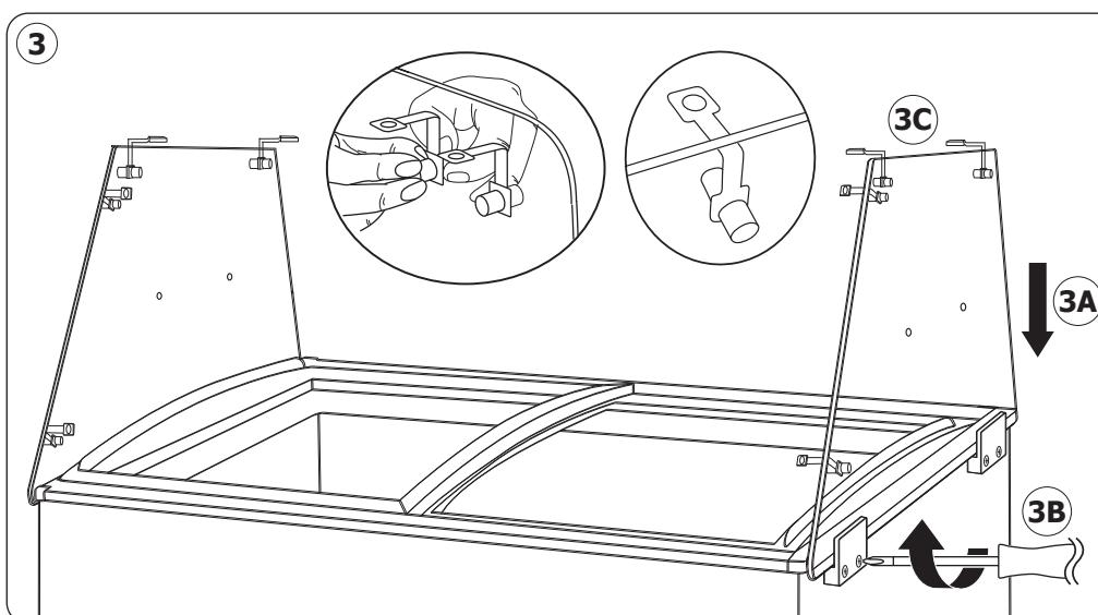
Step 3: Slot the 2 side panels into the clips. Then tighten the clips with screws to fix the side panels in place.
