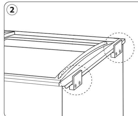
Step 2: Install the glass fixing clips. Do not tighten the clips at this stage.
