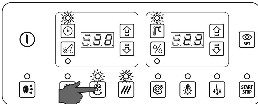
Pressing autoreverse button, shown on the side, the corresponding led switches on to indicate that the function is active.
