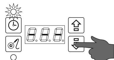
In this case, while cooking the time display will show how long the cooking process has started (instead of showing the missing time to end the process).
