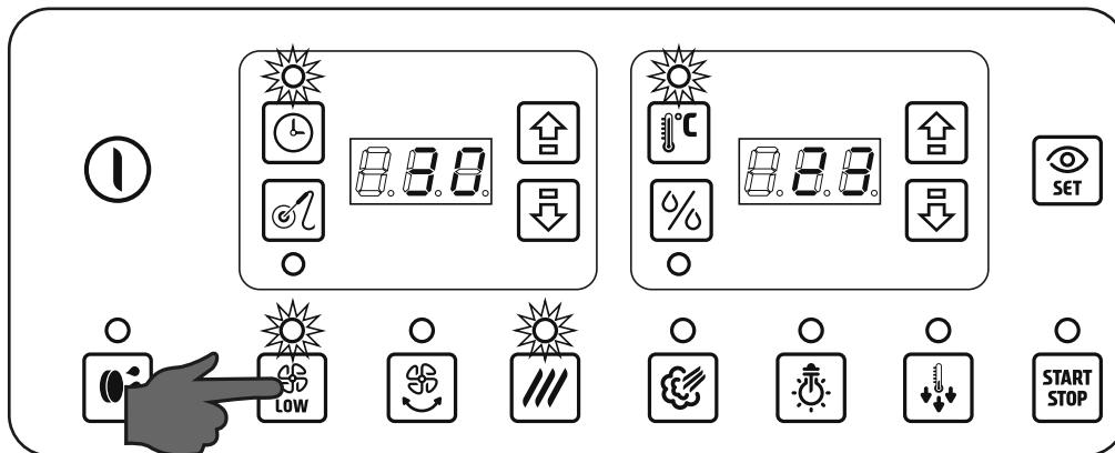
Pressing the reduced ventilation button, shown on the side, the corresponding led switches on to indicate that the function is active.
