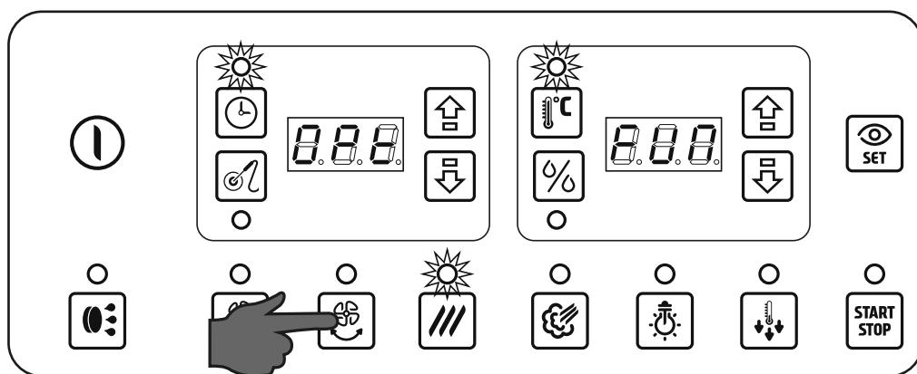
If you didn't buy these functions along with the oven, pressing one of the Autoreverse or reduced ventilation button, the display will show the message **Fun OPT** (function optional) to indicate the selected function is an optional, that is not installed on the oven.
