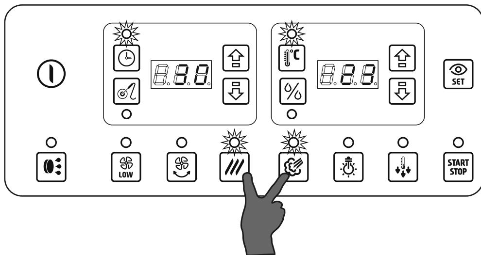
As we explained in the previous paragraph, at the first lighting of the oven, the panel will show convection mode and the default parameters.
