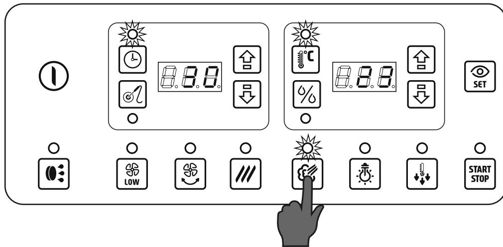
To select steam mode, press the button shown upside. When the led above the button is on, this confirms the selection.
