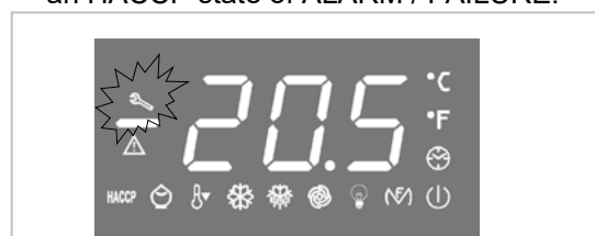
THE LED lights require cleaning of the condenser filter.
