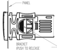
The instruments shall be mounted on vertical panel, in a 29x71 mm hole, and fixed using the special bracket supplied. The temperature range allowed for correct operation is 0÷60 °C. Avoid places subject to strong vibrations, corrosive gases, excessive dirt or humidity. The same recommendations apply to probes. Let air circulate by the cooling holes.
