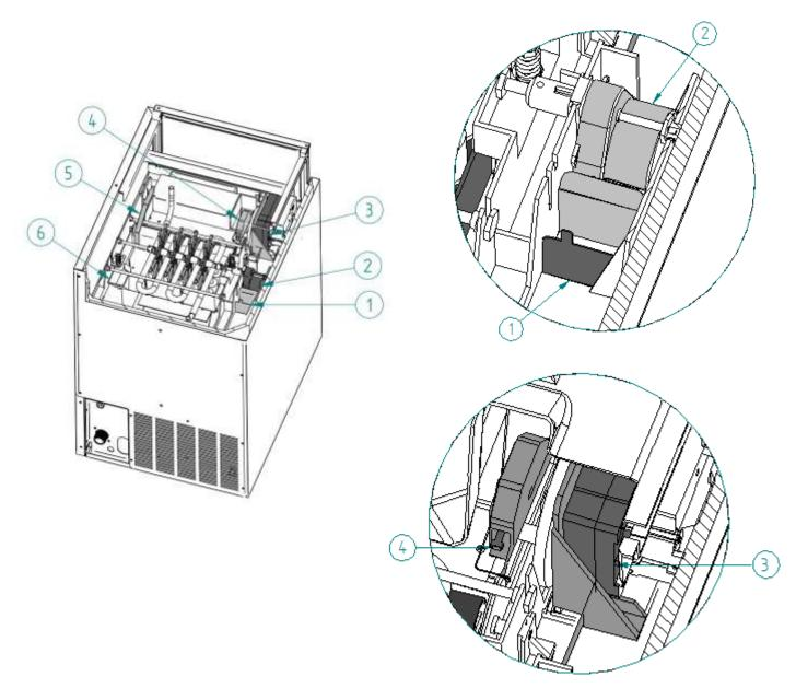
Then, the production time starts, and the ice cubes start to shape in the evaporator until the paddles touch the ice, tilt the motor and contact the Paddle Micro-Switch (EA) plate. Then the Paddle Motor (A) stops and the Pan Cam Motor (V) and the Hot gas Valve (GC) starts, making the harvest cycle begin.
