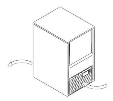
In case the front louver is not enough, the exit is either total or partially obstructed or due to its placement it will receive hot air from another device, we recommend, in case it is not possible to change the location of the machine, TO INSTALL A WATER CONDENSER.
