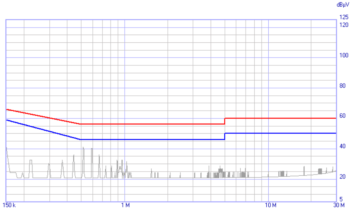
Figure 3: Trend of the disturbance on L2 power conductor See table below for highest peaks characterization
