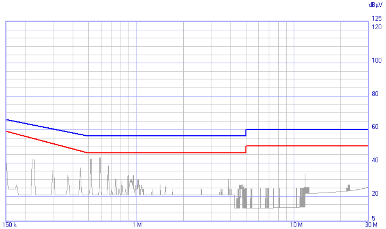
Figure 4: Trend of the disturbance on L3 power conductor See table below for highest peaks characterization
